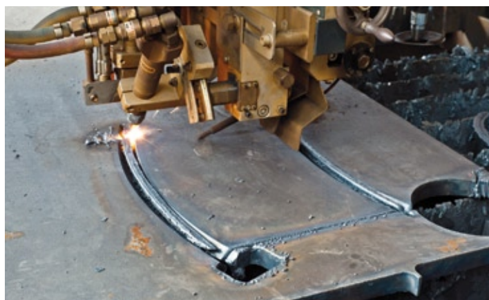
Testa bevel 3 cannelli oxy • 3 torches oxy head
