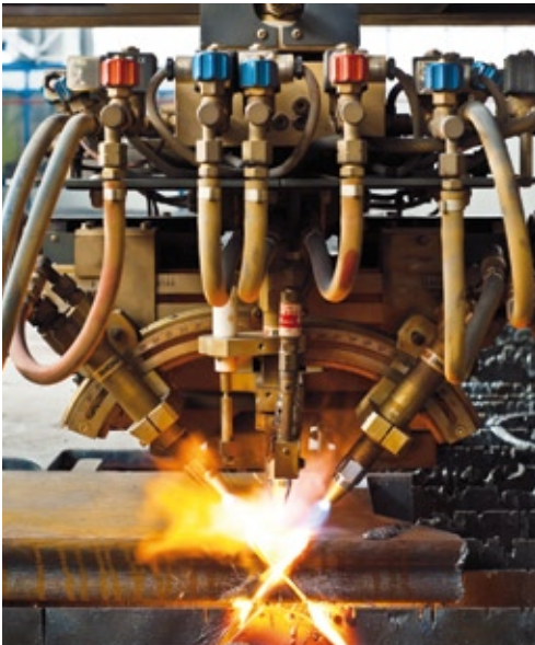
Testa bevel 3 cannelli oxy • 3 torches oxy head
